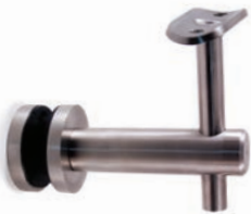
AISI 303 AISI 316 Description S E022/S2 E022/S2316 For glass thickness 5/16" - 7/8" Glass to be drilled at 55/64" dia.
