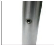
1 Drill and thread M8
