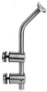
AISI 304 AISI 316 Description S E035300 E035300316 For glass thickness 5/16" - 1" Glass to be drilled at 19/32" dia.
