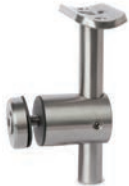
AISI 303 AISI 316 Description S E035200 E035200316 For glass thickness 5/16" - 7/8" Glass to be drilled at 19/32" dia.
