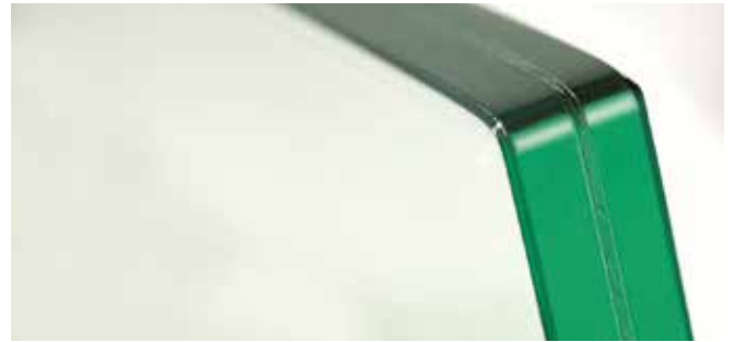
Dettaglio di vetro composto da due lastre alternate da un intercalare in materiale plastico. Glass details are composed of two layers, which are alternated to plastic materials
